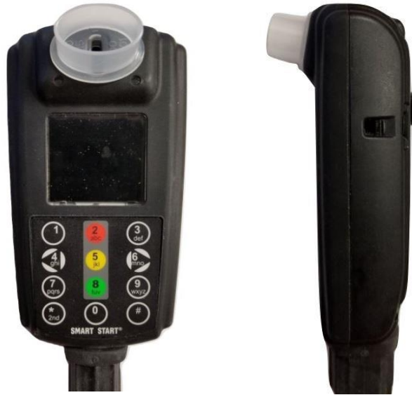
Figura 4 Maayos na Naipasok na Mouthpiece
