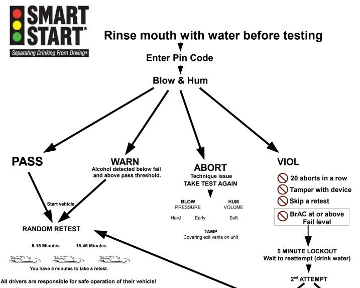
Horn will sound and lights will flash if you MISS or FAIL a rolling retest, or DISCONNECT handset with vehicle running.
